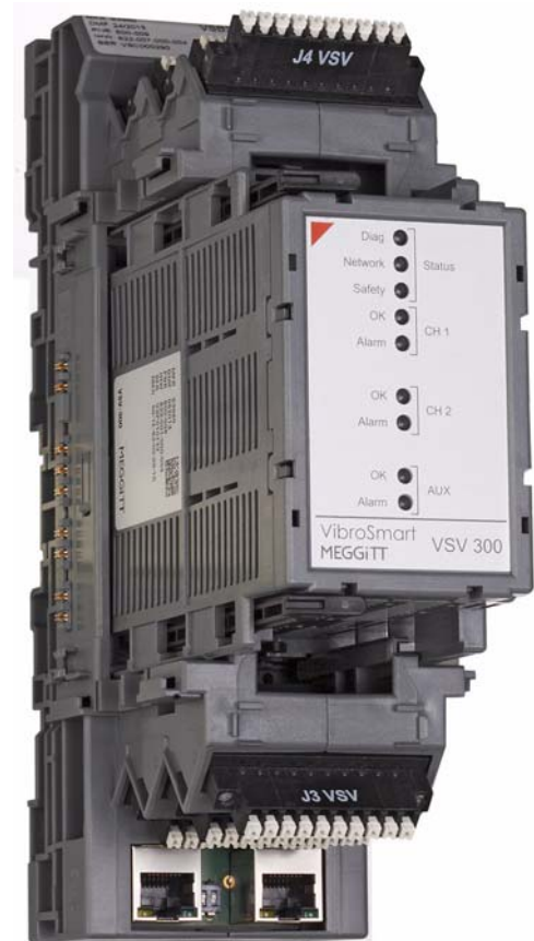
VSV300 vibration monitoring module (mounted on a VSB300 terminal base)
