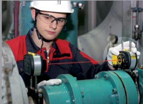
Adjustment of the laser beam The four adjustment LEDs make centring the laser beam child's play.
