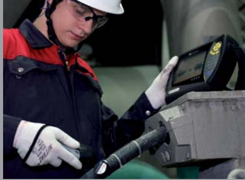
Identification of the machine Use the RFID reader for clear identification of machine to be aligned – all at the press of a button.
