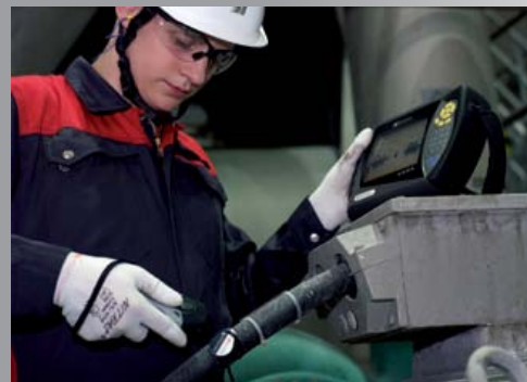
Save Updated machine data and alignment status are recorded on the RFID tag.
