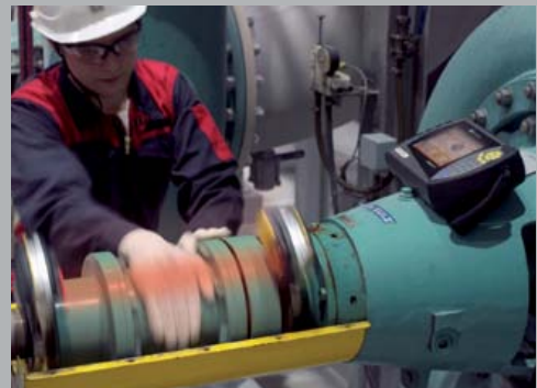
Measurement Hundreds of measurement points are collected and transmitted wireless to the computer.
