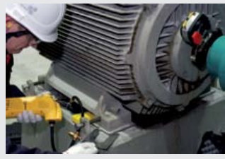
Optional: shims (left) and a lifter unit to lift machine to insert or remove shims.
