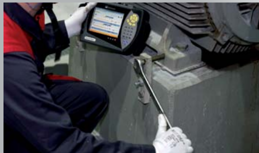
Vertical and horizontal alignment correction Simultaneous live monitoring of machine corrections in vertical and horizontal directions. PERMABLOC® shims in appropriate sizes simplify the process of raising or lowering the machine.
