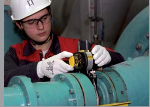
Mounting Sensor and laser mounted on the shafts using the compact chain type bracket or the magnetic bracket.
