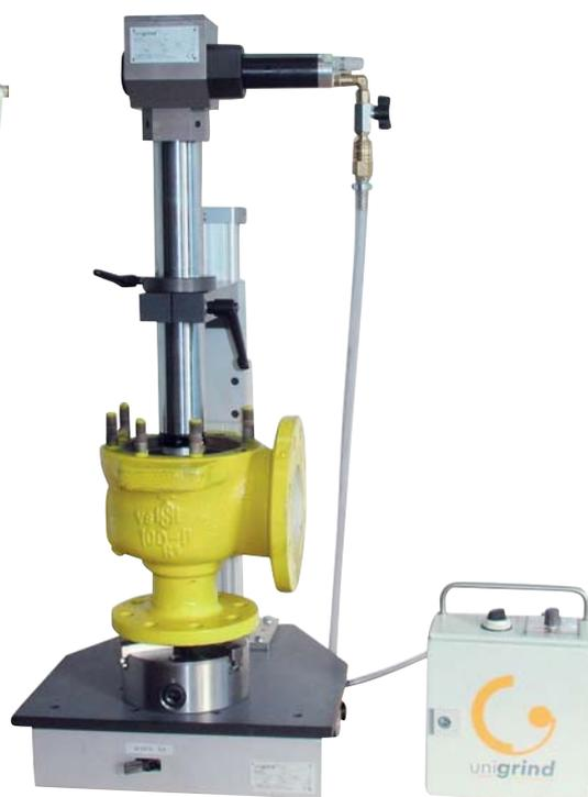
SVS 1 grinding a valve on machine stand
