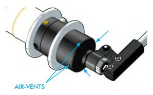
The TFA15TI uses a hydraulic cylinder to advance the Alignment Piston and align the flanges. The hydraulic pressure is applied using the integrated hand pump, enabling accurate control of the force applied.
