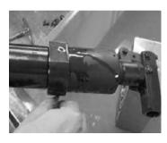
Replenish any missing hydraulic oil by pouring into the Oil Fill hole until excess spills over (middle photo).
