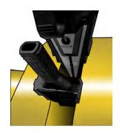
To use the next smallest step, actuate the wedges to around 75% prior to inserting back into the joint. Place the tool in the gap and actuate enough to relieve the load on the Safety Blocks. In this way the flange joint can be progressively closed.
